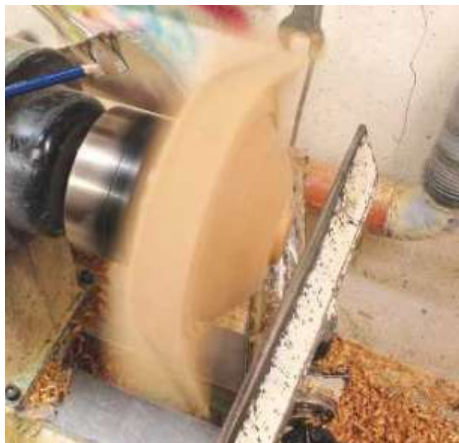
▲ Pic.10 When you draw a thick line (as I have done here) you can see it when the lathe is spinning. The bevel of the tool will need to follow this line around in order to give you the desired shape
